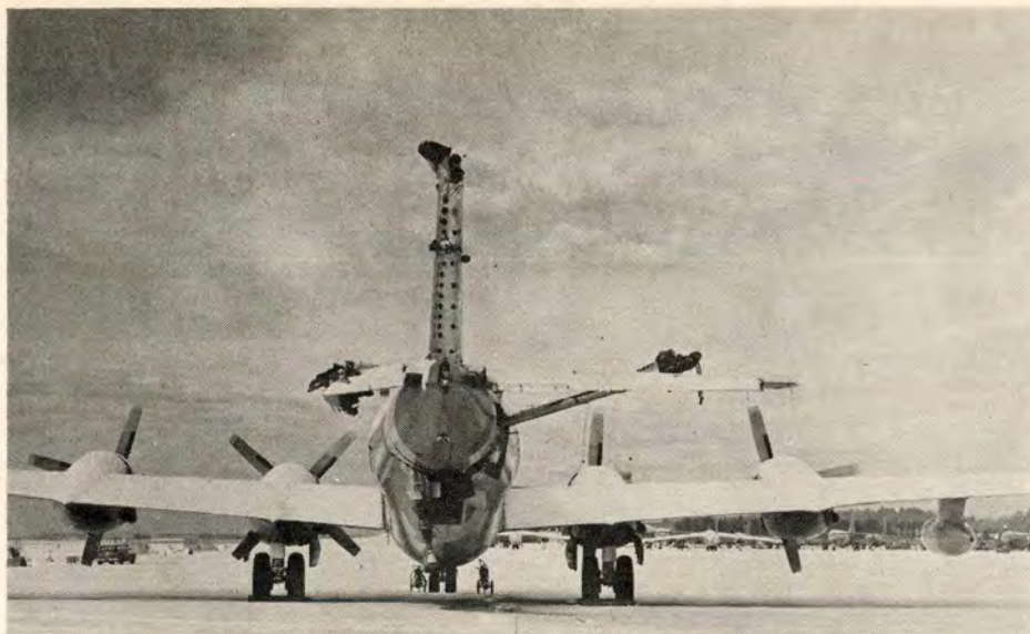
The accompanying photographs show damage to the tail section of an Air Force tanker that had been involved in a midair collision with a receiver aircraft during inflight refueling operations.
